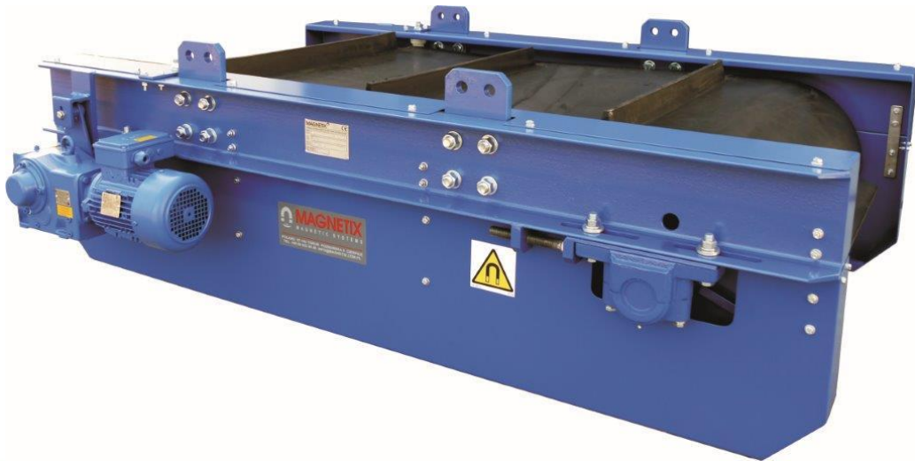
Picture above represents a magnetic separator which captures ferrous metal
